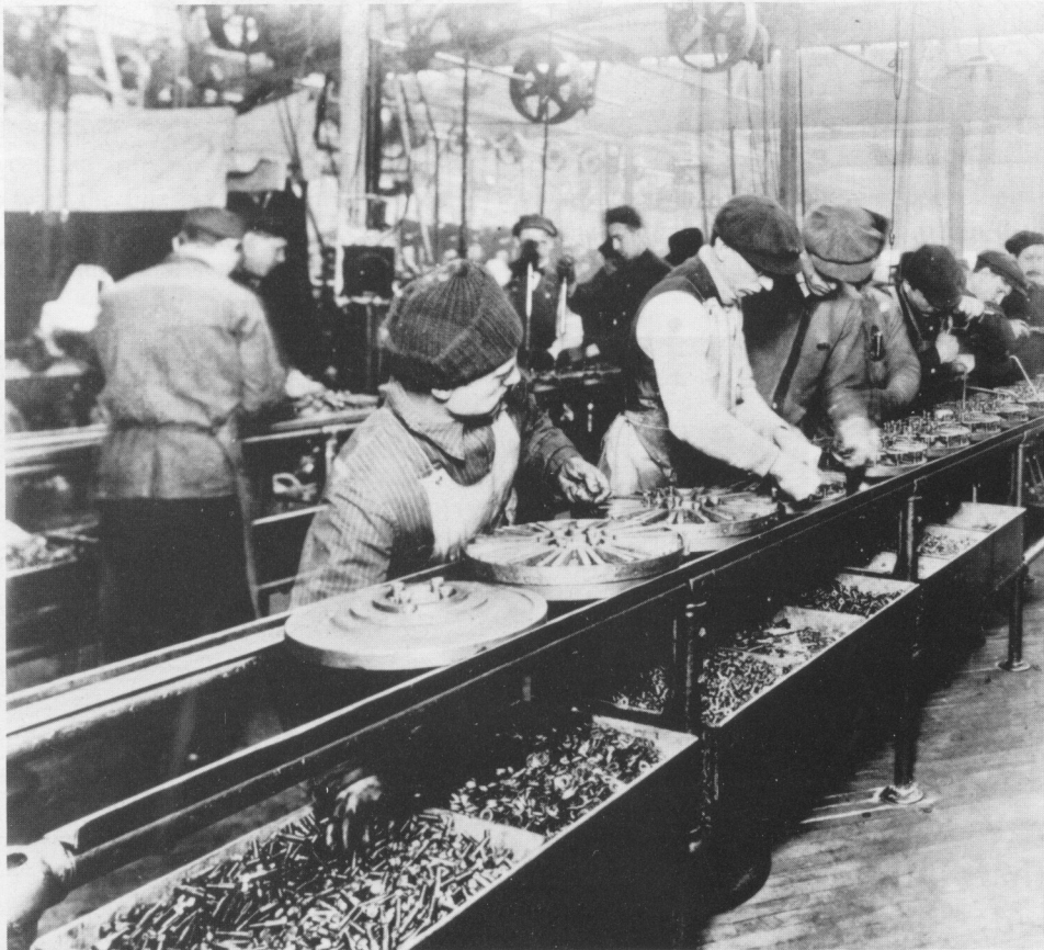
Pass it on: employees at Ford's Highland Park (Michigan) plant on the first automotive component assembly line (1913). [Ford of Canada Archives]
