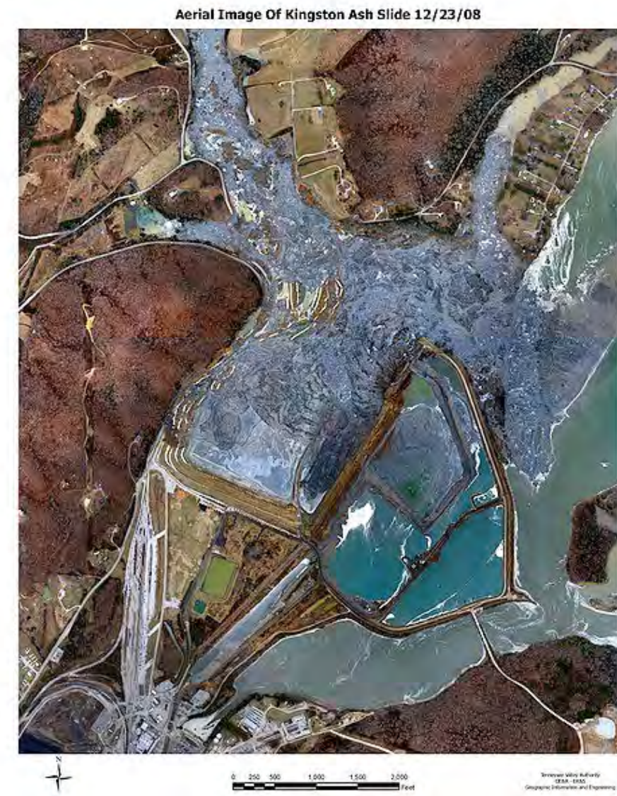
Aerial image of a coal fly ash slurry spill in Kingston, Tennessee, taken the day after the spill in December 2008
