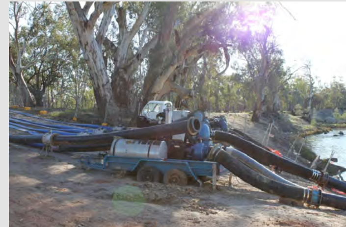
Pumping Machinery to bring water from the River Murray to flood wetlands in the Hattah Kulkyne National Park, July 2009
